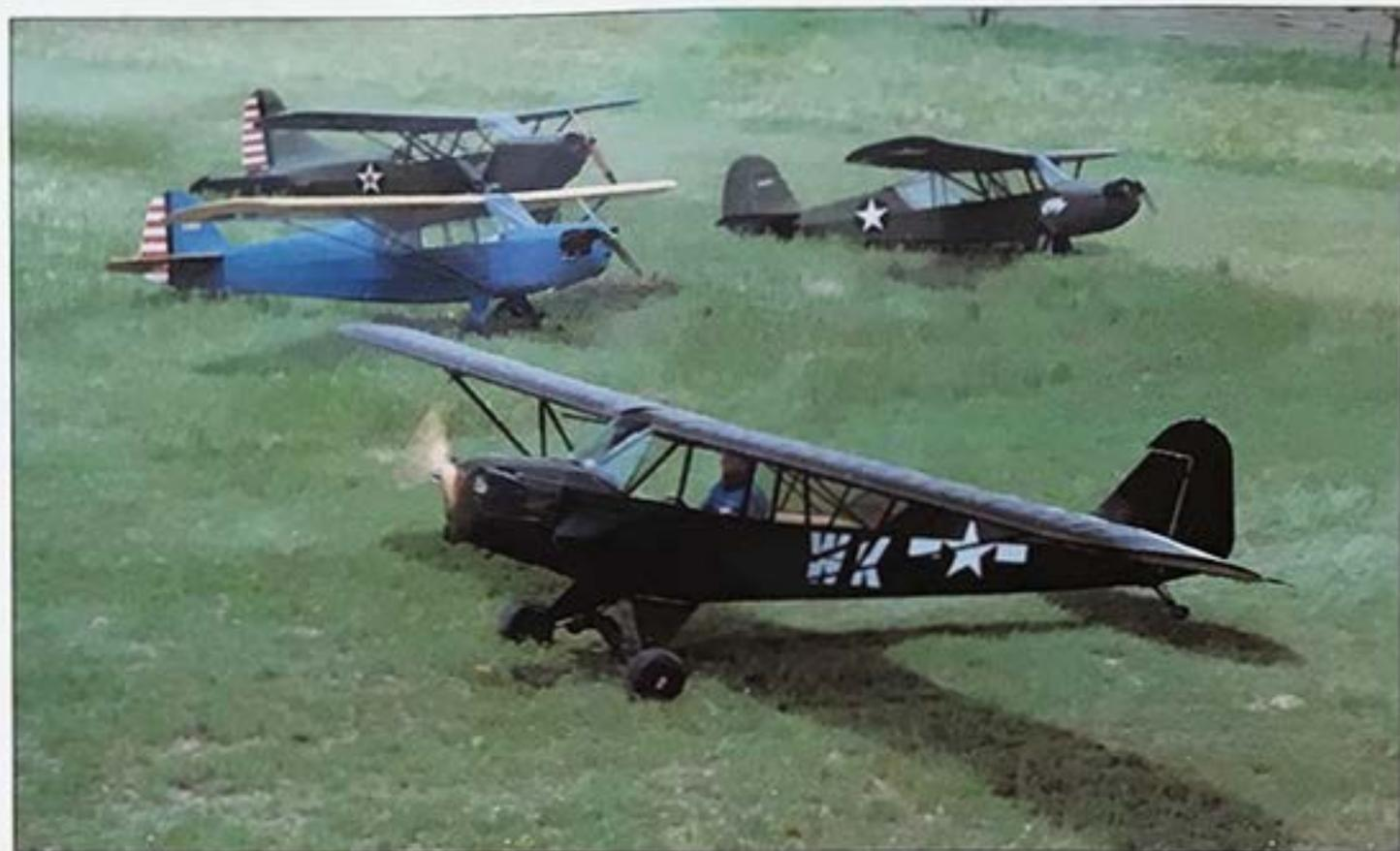
From front to back, an L-4, L-2, L-3 and an L-5. Sometimes known as "Grasshoppers," these versatile ships could take off and land on virtually any "semi-flat" surface.
